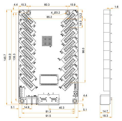
Tolerance: ±0.3 Unit: mm
