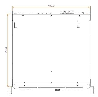
Tolerance: ±0.3 Unit: mm
