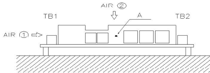
\* Please make air flow to maintain the heat sink (part A) temperature 85°C or less (Operating ambient temperature is 50°C ).
