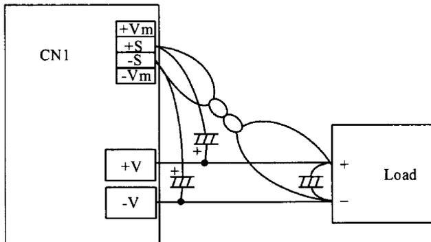
When the function of remote sensing is not in used, connect +S terminal to +Vm terminal, and -S terminal to -Vm terminal by the attachment connector.
