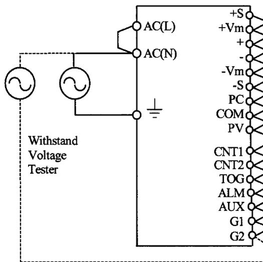
Output ~  $\perp$  (chassis) : 500VAC 1min. (100mA),
