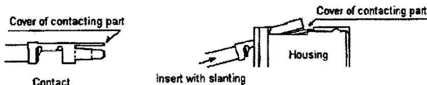
**d). Mating and Unmating Connector**
