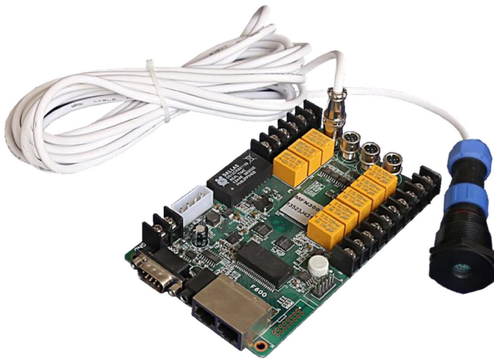
Figure 1 Connection between NS060 and MFN300 multifunction card
